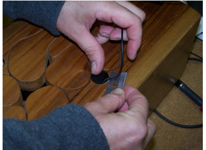
2. Carefully wedge a flat blade (such as a razor blade, thin knife, etc.) between the pickup and the instrument. Again, do not pull the pickup away by its cable.
