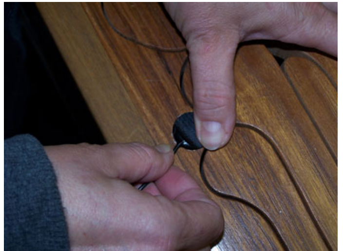
11. Press on with finger, making sure that the whole pickup head is firmly attached to the instrument.
