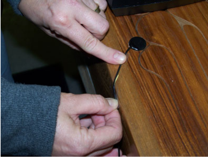
12. Secure the pickup cable with a piece of scotch tape to ensure clean sound transmission.
