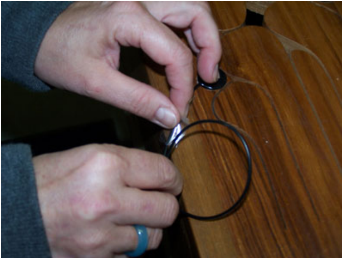
1. Remove any tape that is securing the cable. NEVER pull the cable!
