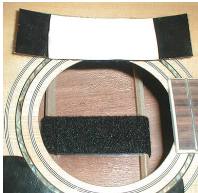
Temporary Velcro attachment for preamp mount
