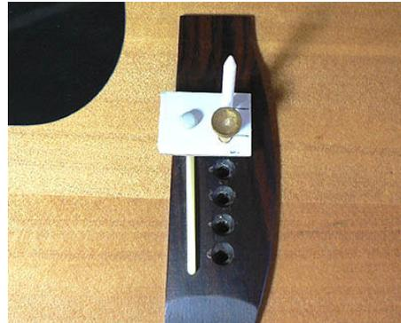
8. Form a putty-ball and place it on the jig over the saddle between the high e and b string.
